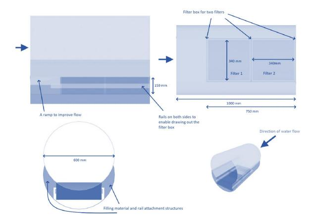
Figure 36 Technical drawings of a horizontal flow filter
