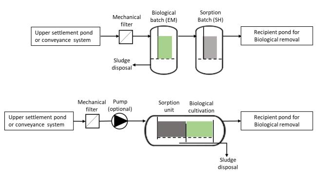
Figure 2 Main SHEM Water Purification concepts.
