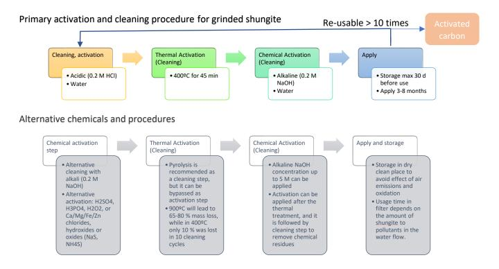
Figure 20 Recommended activation and cleaning procedures for shungite
