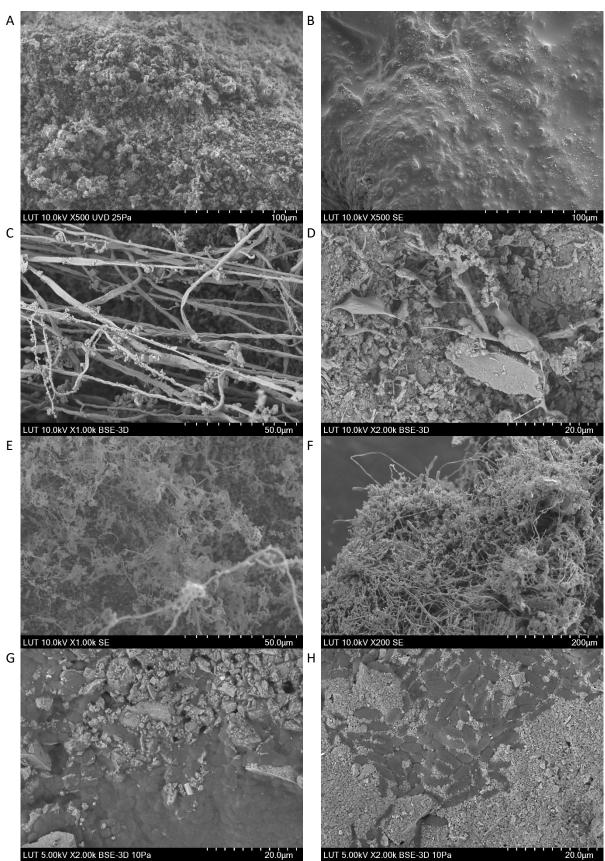
Figure 27 SEM images of microbial growth on surface of shungite rocks after 14 days exposure to EM solution. Collection of SEM images from the EM growing study. a: clean shungite surface, b: shungite surface with a possible biofilm growth on it, c: fibrous growth on shungite, d: possible bacterial growth on shungite, e: fine fibrous growth on shungite, f: fibrous growth on biochar, g: bacterial growth/film on zeobas granules, h: bacteria on ceramic powder.
