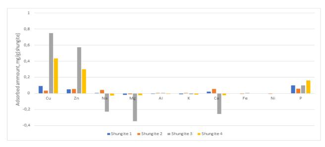
Figure 12 Results from the metals adsorption test of 4 different untreated shungite grades. Results given in mg/g(shungite). Negative bars indicate that the element in question has been released from the shungite during the adsorption experiment.
