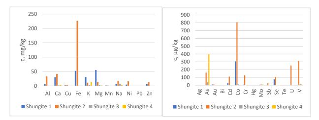
Figure 9 Results of some metals from leaching test (L/S = 10, SFS-EN 12457-2:2002). Inert waste has threshold values for example to Ni (0.4 mg/kg), and Zn (4 mg/kg). Therefore, shungite grades #1 and #2 would not be environmentally feasible in Finland: SH#1 leached 4.5 mg<sub>N</sub>/g, and 6.9 mg<sub>Zn</sub>/g and SH#2 17 mg<sub>N</sub>/g, and 6.9 13 mg<sub>Zn</sub>/g
