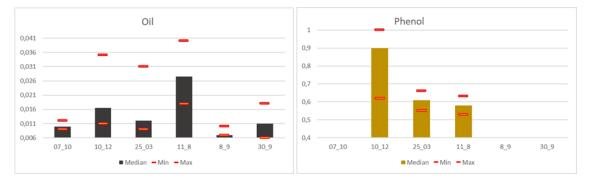
Figure 75 Concentrations of oil products (mg/l) and phenol (μg/l) in the water of Dudergofskoe-Dolgoe lake system.
