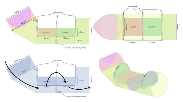
Figure 34 Technical drawings of the vertical flow filter. Filter was applied in Sammonlahti CW in 2020-21 field tests.
