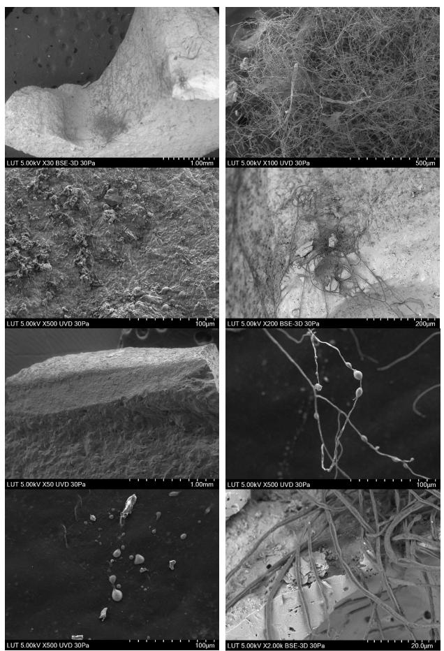
Figure 22 Scanning electron microscope was applied to study the growth of EM. Example SEM images of 10 days cultivated EM on shungite.
