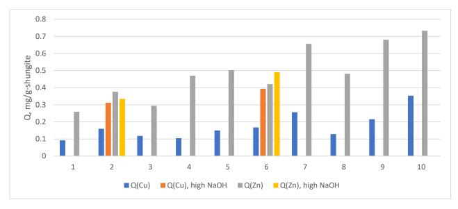
Figure 19 Re-usability: shungite samples from filters were treated chemically with HCl (0,2 mol/L), physically (thermal 45 min, 400 °C) and finally with NaOH (either with 0.2 mol/L or 5 mol/L). After 10 treatment cycles the adsorption capacity was still high or increasing. Mass loss was approximately 1 % in each treatment (total 9 % of shungite was lost in 10 cleaning and activation cycle). The shungite is a durable and stable material.
