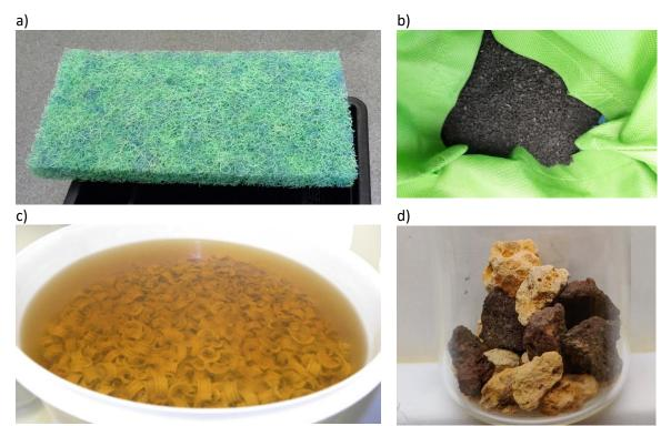
Figure 33 a) foam applied in removal of fine particles, b) shungite were in fiber bags (or geotextile bags), c) EM solution fermenting in laboratory with the ceramics, d) porous lava rocks were studied in field test 2019 as an alternative for ceramics.
