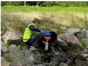
B) Samples from pipe outflow were collected with instruments that allowed the whole profile across the cross flow to enter the sample.
