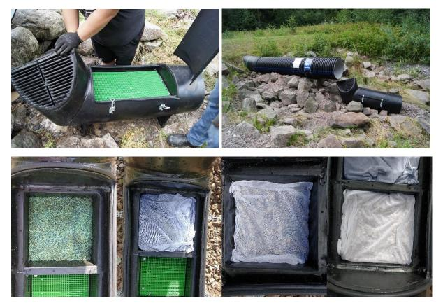
Figure 35 Vertical flow filter applied in Sammonlahti CW at 2020-2021 field test.
