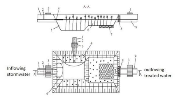
Figure 56 General scheme of the retention pond. 1 -supply ditch; 2 -grate for floating debris; 3 -bridges; 4 -floating boom for absorption of oil products; 5 -buffer pit for deposition of large fractions of suspended solids; 6 -part of the reservoir with aquatic plants; 7 -natural sorbents on the bottom of the pond; 8 -outlet filter with sorbent; 9 -outlet ditch.
