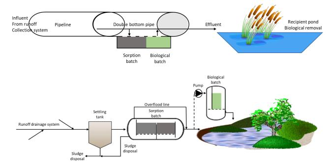
Figure Appendix 3.3 Underground or in-transportation-system solutions. 1) System implemented in pipeline, 2) sorption unit implemented into runoff drainage system and independent biological unit is applied to dose cultivated EM to recipient aquatic system or soil at shore.
