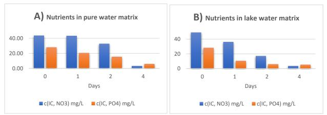
Figure 23 Examples of test results of activation and effect of EM solution in laboratory environment. EM solution is added to artificial nutrient solution prepared to distilled laboratory water or lake water. Results should be visible in 2-4 days as significant decrease in concentration. nitrate concentration tends to decrease slower than phosphate. If lake water or run-off water is applied as matrix, the decrease is faster due to the micro-organisms in the water matrix present.
