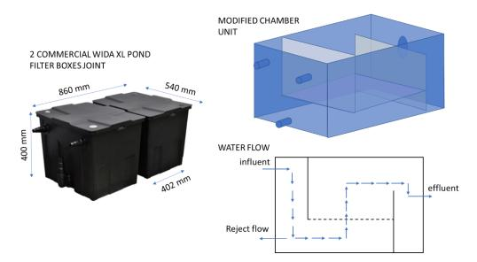
Figure 32 Modified Wida XL boxes were applied in pre-tests of filter media in Sammonlahti constructed wetland in 2019. The boxes were modified from original pond filter systems allowing higher flow rates through two chambers. The first box contained a foam layer and shungite, and second box foam layer and EM in growth media. fine particles were removed from boxes via a reject flow. preliminary filtration to remove large size particles were made with a net installed to water intake.
