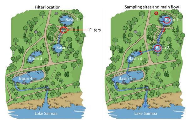
Figure 40 Sammonlahti CW in 2020. Basin 4 was built in 2020. Filters were implemented in 2019 and 2020 at outflow from basin 1. Water quality was monitored as composite samples from Basin 1 and 2, and their out flows.
