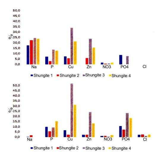
Figure 13 Results from the metals adsorption test. Results given in % in a) high concentration, and b) lower concentration of the metals. Adsorption mechanisms are affected by the ion concentration in the solution (Na). Nitrate removal is inefficient with any shungite fraction studied.
