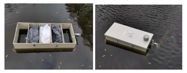
Figure 30. Installation of sorption filter equipped by water pump.
