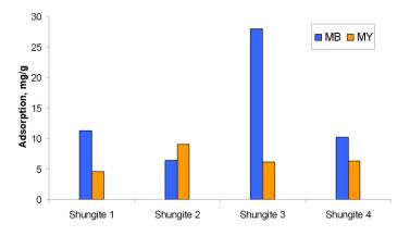
Figure 11 Sorption activity of shungite rocks to cationic and anionic complexes on the example of methylene blue (MB) and methanyl yellow (MY) for shungite 1, 2, 3 and 4. The method can be applied in selecting potential shugite grade. The methodology is novel Raman based analytics and published by SHEM-WP project partner (Rozhkova & Kovalevski, 2019)
