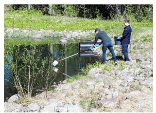
A) Sammonlahti Basin 1 and 2 water samples were taken as composite samples of 5-10 subsamples. The depth of water was typically 50 +/- 20 cm.
