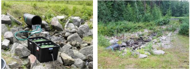
Figure 42 Pre-test filter located at outlet of 1st basin at Sammonlahti constructed wetland
