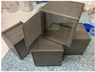
C) Microplastic analyses: metal cages were filled with shungite and placed in filters for a month. Mesh 2 mm.
