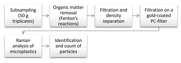
Figure 88 Microplastic analyses: sample treatment for Raman analysis is a multistep process that contains several extraction and filtering steps. To avoid contamination special instruments and laboratory hoods have to be applied.
