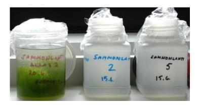
Figure 24 Examples of run-off water samples applied in testing EM. Presence of EM boosted samples containing algae more than samples without visual algae growth. Bacteria on Green filamentous Algae is expected to have a significant role in nutrient removal and laboratory results supported the assumption. Results reported in this chapter are gained from water samples without visually clearly seen biomass (similar to samples 2 and 5).
