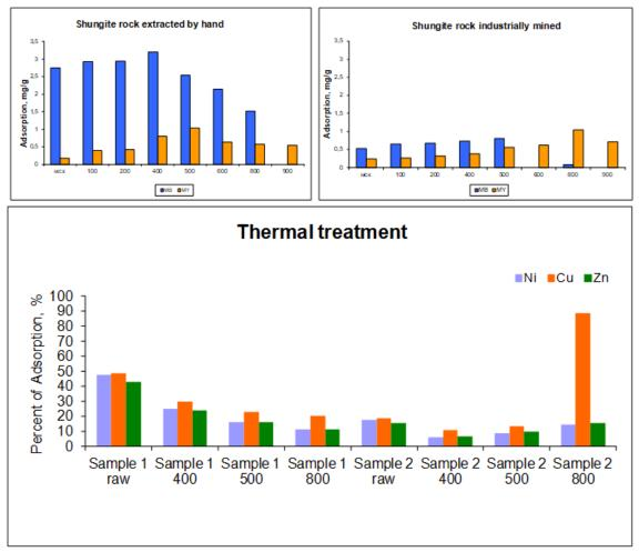
Figure 17 Effect of thermal treatment on adsorption (Kovalevski, Reinikainen, Reinikainen, Rozhkova, & Sihvonen, 2020)
