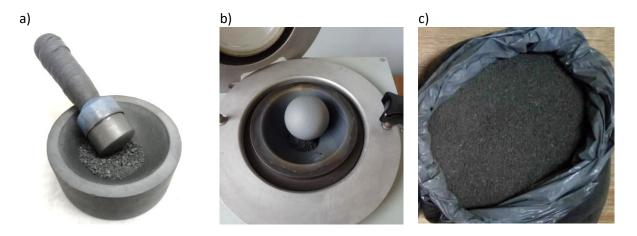
Figure 6 A) Crushing by abrasion (agate mortar), B) Crushing by splitting up (vibration impact mill), C) Shungite after crushing.
