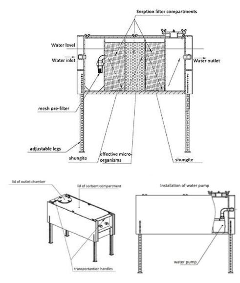
Figure 29 General scheme of sorption filter.
