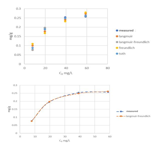
Figure 15 Adsorption isotherm models computed for Zn adsorption and comparison to measured experimental data of shungite samples. The isotherms, namely Langmuir-Freydlich isotherm reveals that the adsorption energy is normally distributed on the surface when treated with alkali (0.2 mol/L NaOH). NaOH seems to make the surface more hydrophilic, which allows metal components closer to the surface increasing the reactivity. (Potila, 2020)
