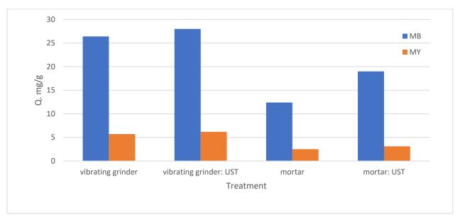
Figure 8 The adsorption capacity (for the removal of MB and MY) of SH samples crushed with mortar, and in a vibrating grinder: Before and after ultrasonic treatment (UST).
